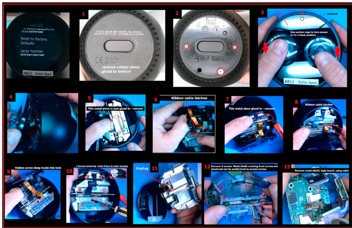
Fig. 4. Step-by-Step tear-down of Amazon Echo Spot.
